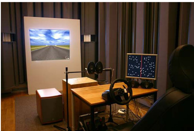
Figure 1. Driving simulator in a sound recording studio with the projected driving scenario (4 m in front of the subject), secondary task (1 m, approximately 45° to the right of the subject) and loudspeaker setup.
