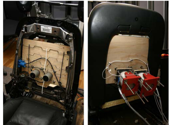
Figure 4. Mounting of shakers in the back of the driver seat for presenting vibrotactile signals to the subject. The seat padding and upholstery were in place during the experiment.
