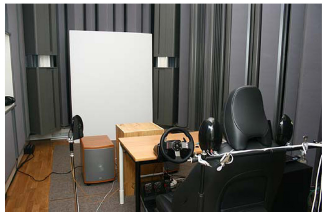
Figure 2. The driving simulator in a sound recording studio with the projected driving scenario (3.7 m in front of the subject), visual and auditory indicators and the modified driver seat with vibration generators.
