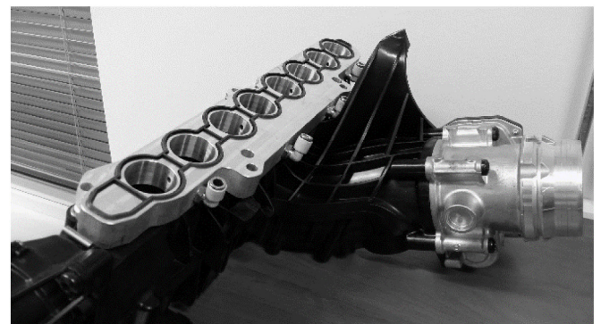
Figure 1. Adaptor plate for CNG injectors attached to intake manifold. Each injector supplies CNG to two different ports (one injector per cylinder)
