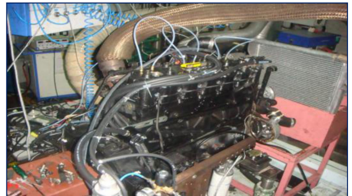
Fig 4. Typical Dual Fuel Engine on Engine dynamometer
