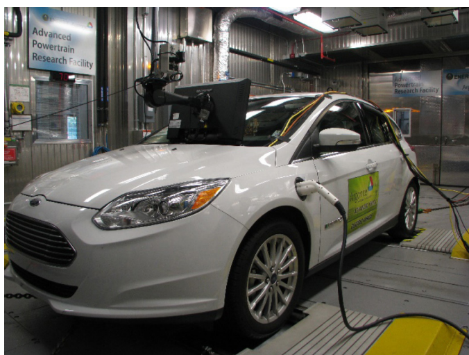
Figure 4. 2013 Ford Focus BEV test vehicle on Argonne's APRF dynamometer for testing.
