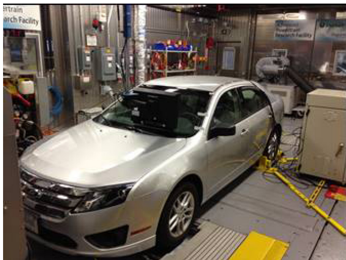
Figure 3. 2011 Ford Fusion test vehicle on Argonne's APRF dynamometer for testing.
