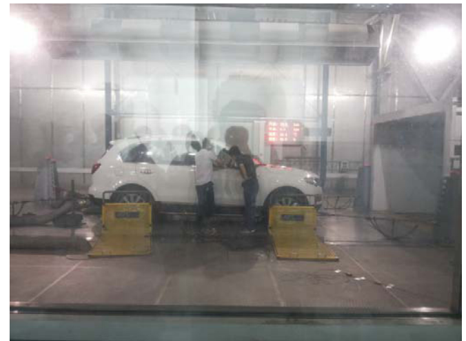
Figure 3. Test vehicle in wind tunnel
