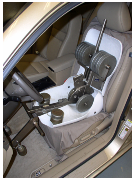
Figure 1. J826 H-point manikin installed in a vehicle.
