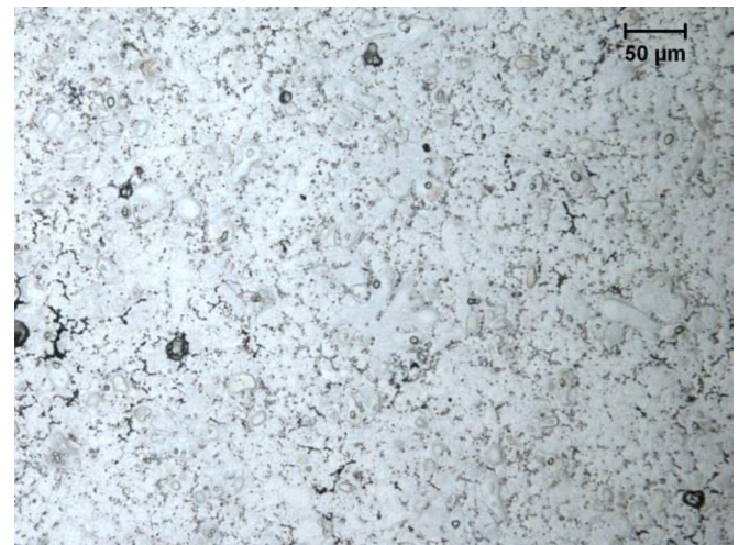
Figure 4. Presence of externally solidified grains in AM60 samples
