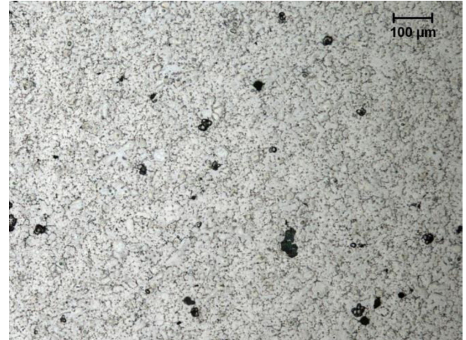
Figure 3. General porosity distribution in AM60 samples
