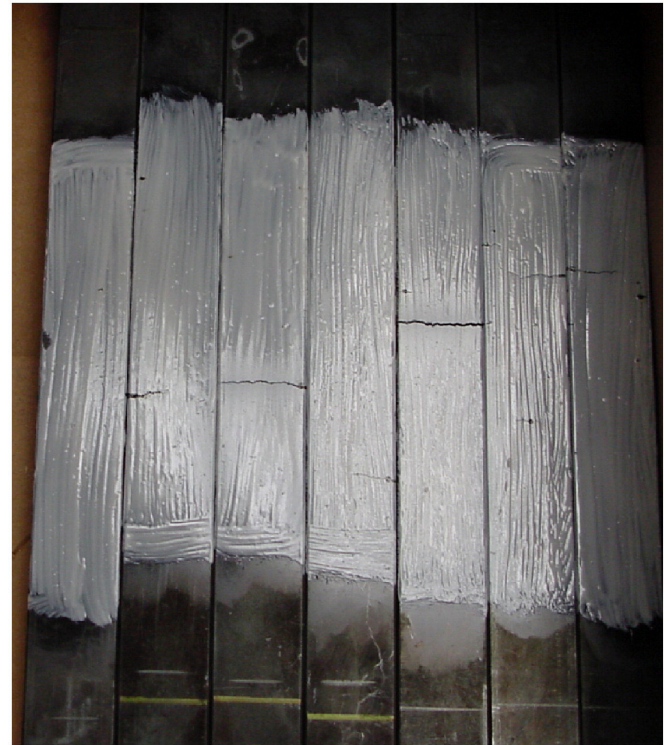
Figure 7. Stress-relieved LRB samples after fatigue tests with applications of ZnO paste.
