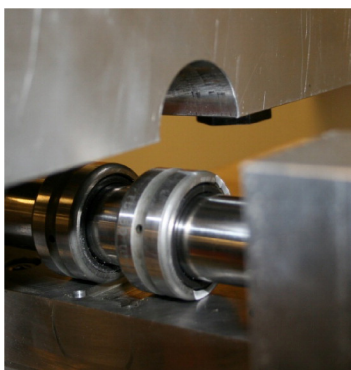
Figure 1. Schematics of (a) the experimental setup for rolling a rectangular bar, (b) a rectangular bar, (c) a front view of the experimental setup, and (d) a close-up view of the roller.
