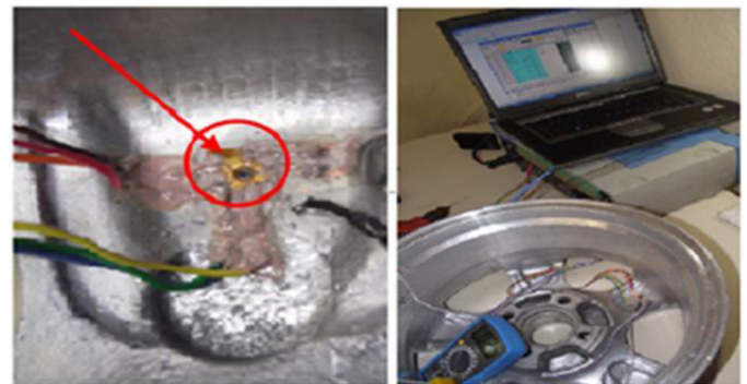
Figure 3. Hole drilling method experimental sequence of trial. The images show the rosette and the arrow points to the center mark.
