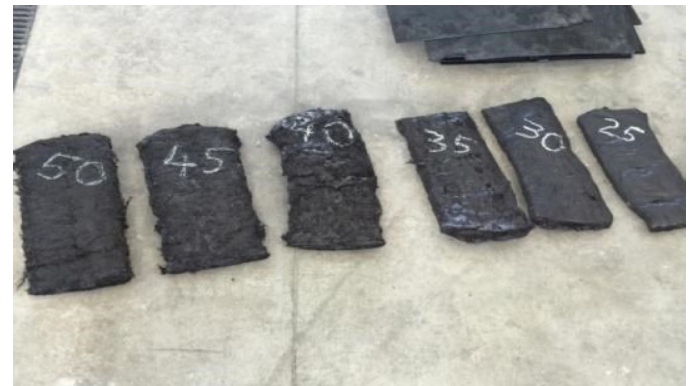
Figure 3. Charge produced by LFT-D prepared for the press.
