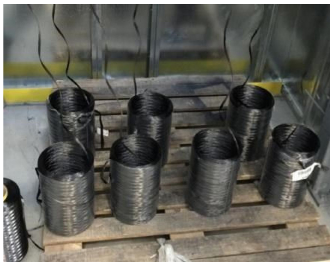
Figure 2. Carbon fiber in rovings prepared for LFT-D feeding.
