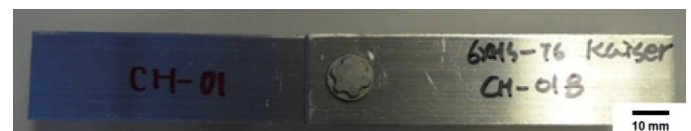
Figure 1. A top view of a lap-shear specimen with a FDS joint with clearance hole.
