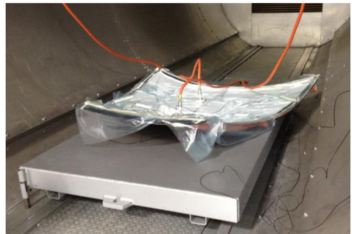
Figure 6. Vacuum bagged mold with carbon fiber lay-up in autoclave.
