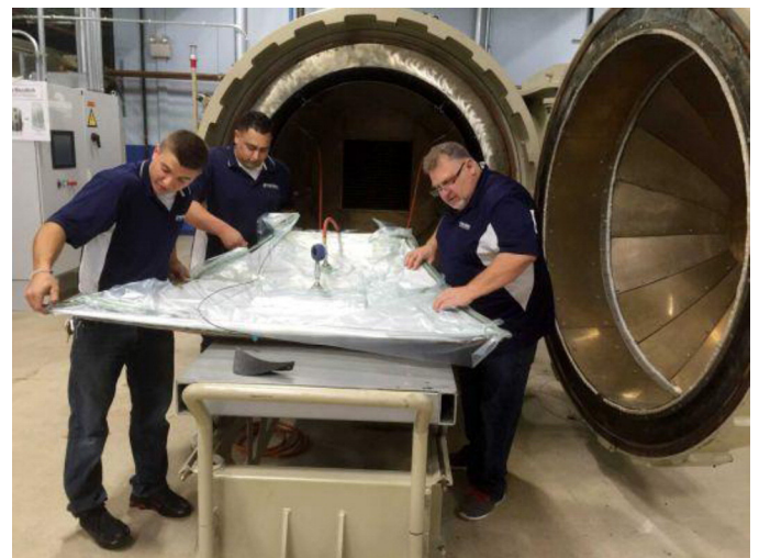
Figure 7. Vacuum bagged mold being taken from the autoclave.
