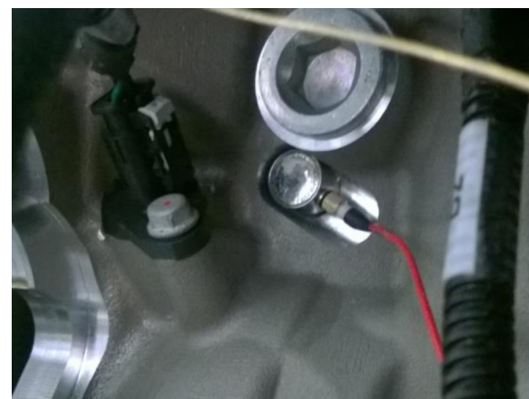
Figure 3. Photograph of the large acoustic emissions sensor mounted at the base of cylinder 4
