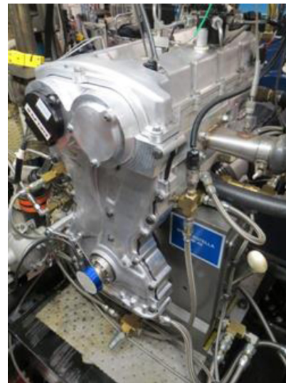
Figure 1. Photo of the Gen 2 GDCI Single-Cylinder Engine Installed in the Delphi Test Cell.
