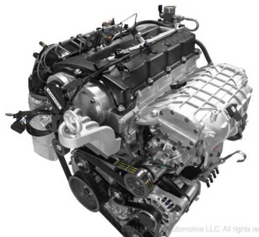
Figure 2. Photo of the Gen 2 GDCI 1.8L multi-cylinder engine (front view).
