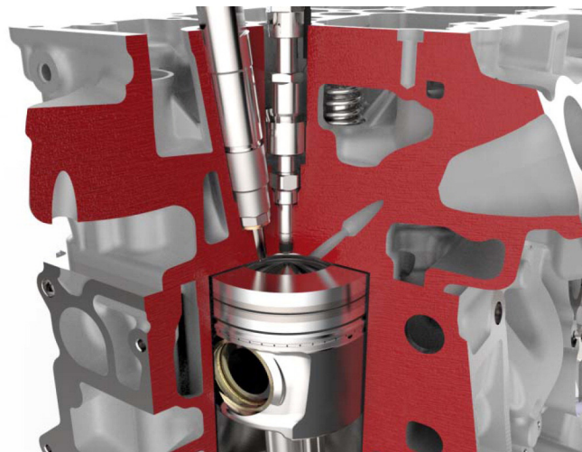
Figure 6. Layout of the combustion system in TDC with the central CNG injector and the inclined diesel injector.
