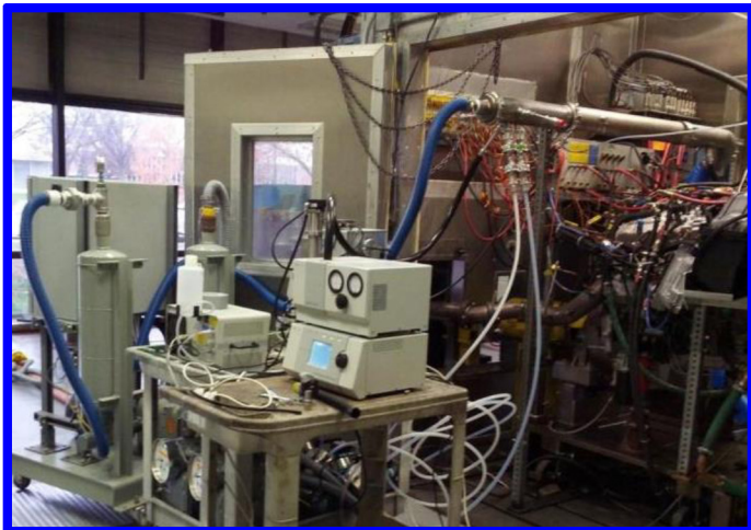
Figure 1. Photograph of aerosol sampling apparatus installed in an engine cell.
