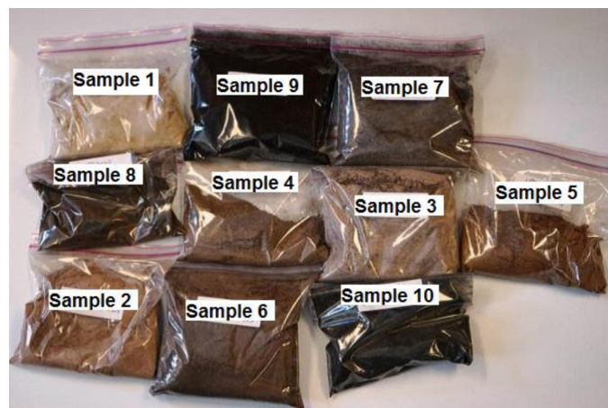
Figure 1. Ash samples as-received from DPF Cleaner.
