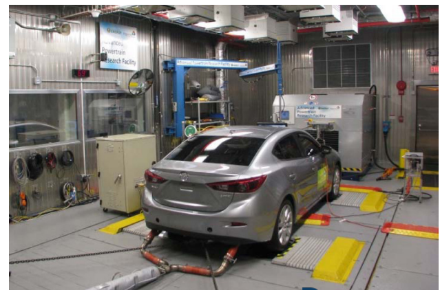
Figure 2. Vehicle during Chassis Dynamometer Testing at Argonne National Lab's Advanced Powertrain Research Facility
