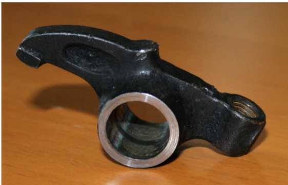
Figure 2. Similar rocker arm design. [7]
