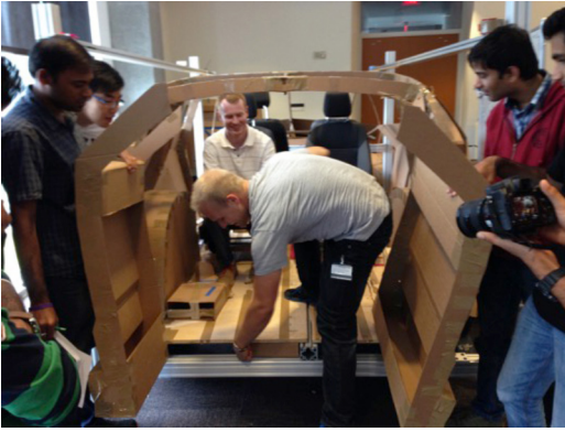
Figure 8. Evaluation of low load floor cargo loading and closure concept
