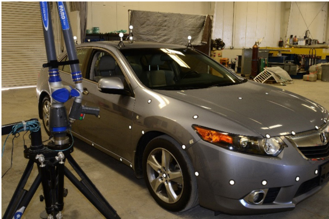
Figure 5. View of the targeted Acura and FaroArm.
