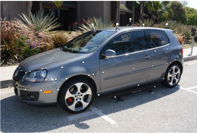
Figure 2. Photograph of the targeted 2007 Volkswagen GTI, illustrating placement of disc targets, spherical targets, and scale bar.
