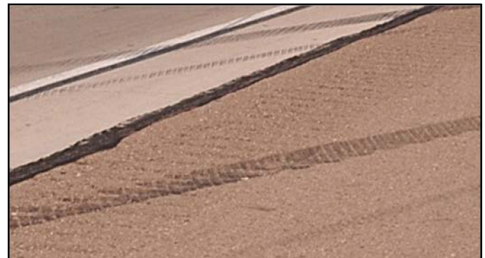
Figure 1. Striated tire marks deposited by a yawing vehicle.
