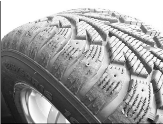
Figure 2. Shoulder block wear as a result of yaw testing.
