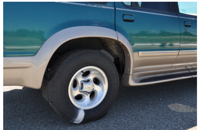
Figure 4. Three hump “lumpy” tire on the right rear position of the Ford Explorer
