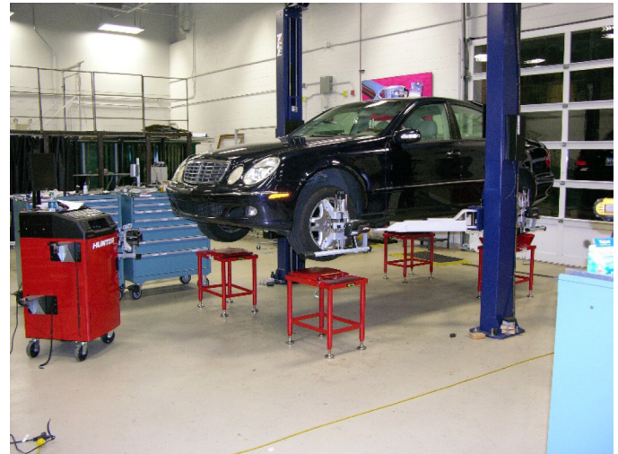
Figure 3. Vehicles are then raised, the heads are attached and compensated, (vehicle V2) and then raised again and lowered for every alignment measurement test.
