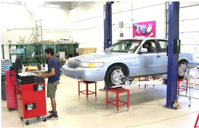
Figure 4. The luxury RWD sedan performing a caster sweep (vehicle V5)
