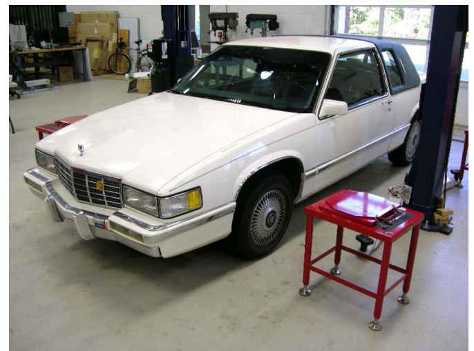
Figure 5. Vehicle bushings underwent large binding forces due to lateral suspension scrub on droop so one protocol was to back cars out of the shop quickly (vehicle V4)
