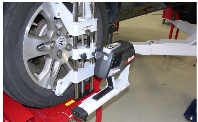
Figure 2. The “DSP700” alignment heads were attached to the wheel rims and compensated for angular errors prior to each test session (vehicle V3)
