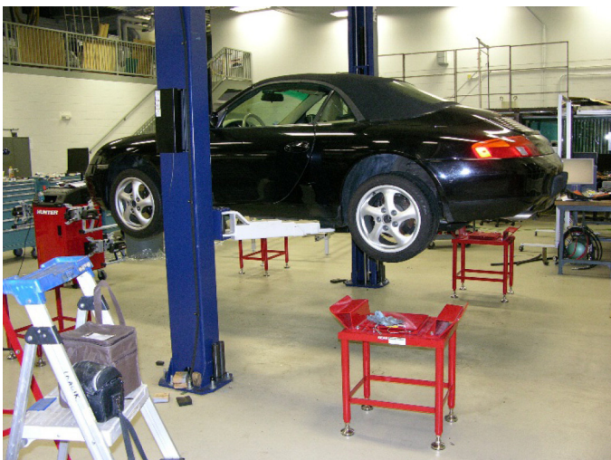
Figure 6. At the end of testing, the vehicles were raised, the heads removed, the bearing plates and stands backed away, and here, vehicle V6 is ready to be lowered to the ground.
