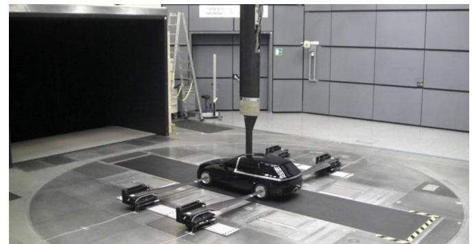
Figure 3. 40% DrivAer wind tunnel model (with estate back rear end installed) inside the AAWK.
