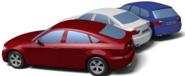
Figure 1. DrivAer geometry with three different rear ends: fast back (red), notch back (white) and estate back (blue) - as introduced in [14].
