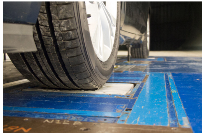
Figure 4. Close-up view of a LDV wheel and GESS wheel roller in the NRC 9 m Wind Tunnel.
