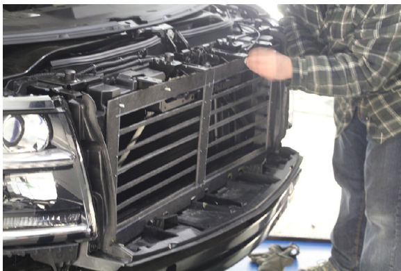
Figure 6. View of the mock-up AGS frame covering the radiator of a standard SUV, front bumper removed.
