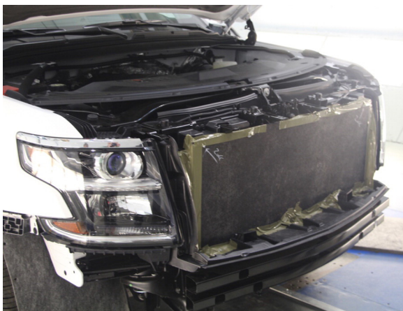
Figure 5. View of the solid panel covering the radiator as part of the custom AGS of a standard SUV built for the study, front bumper removed.
