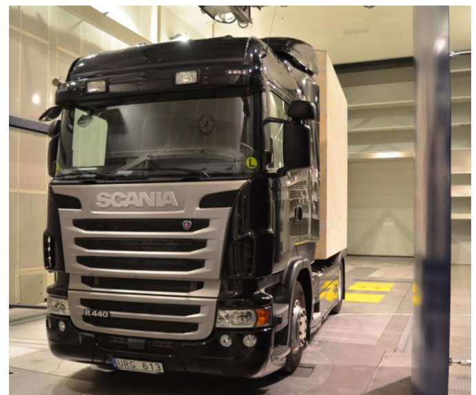
Figure 10. FCD (black) on right side of photo in “backward” position at the front of a truck at yaw.
