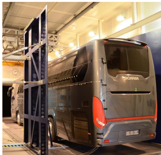
Figure 7. Flow Control Devices (FCDs in black) positioned at 2.2m from the side walls near the rear of the bus. Pressure taps visible at z = 2.5 m. The bus engine inlet is visible at the lower rear corner, on the side of the bus.
