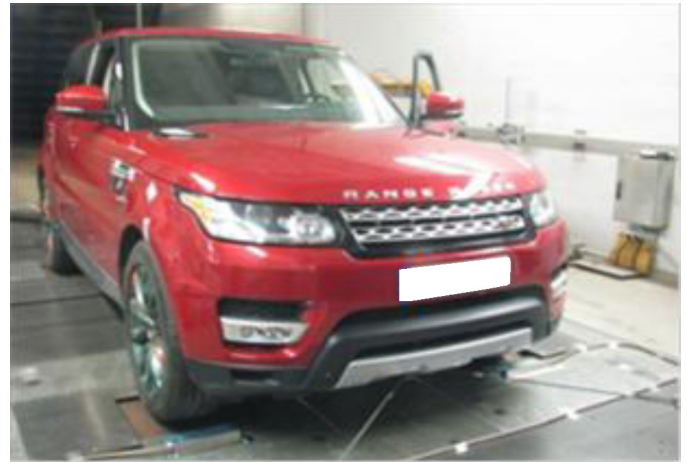
Figure 2. Test Vehicle Setup on the Dynamometers at the FKFS Thermal Wind Tunnel
