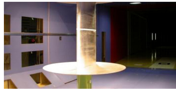
Figure 2. Strip Tube on NACA0012 wing.
