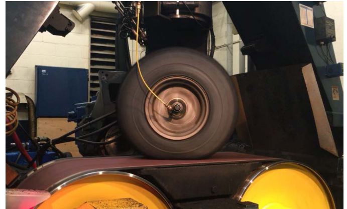
Figure 4. ROV tire on Flat Trac III tire test machine at Smithers RAPRA.
