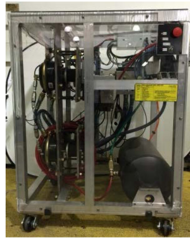
Figure 3. NHTSA Heavy Truck HiL System - Trailer
