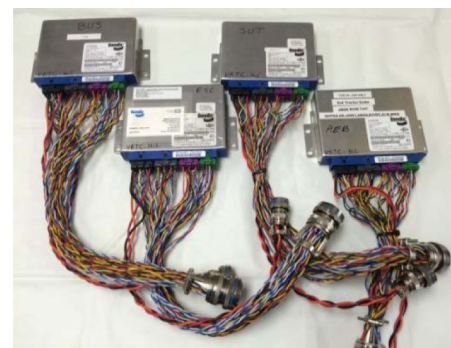
Figure 11. Various ECU-60s with modular quick disconnect
