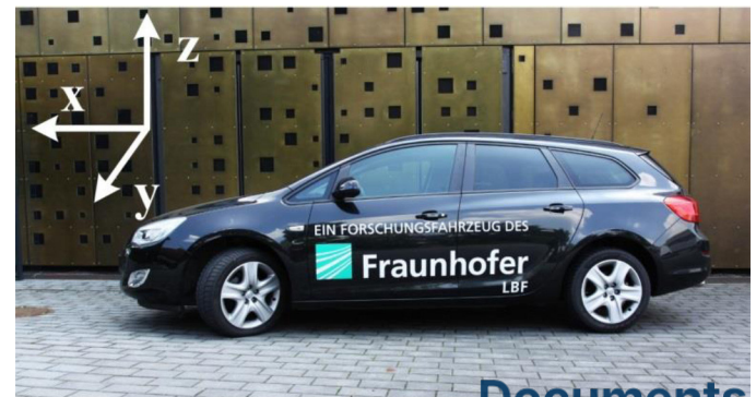
Figure 4. Test vehicle Opel Astra Sports Tourer and associated coordinate system.
