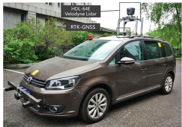
Figure 3. Velodyne HDL-64E and RTK-GNSS product in Touran Test Platform
