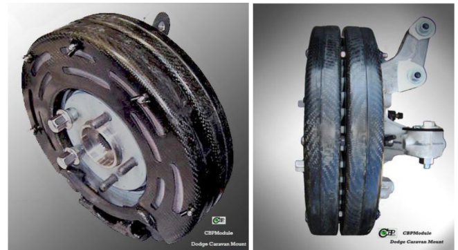
Figure 1. The Brake Pad Waste Collection System as mounted to the knuckle assembly. Left - general view, Right - side view.
