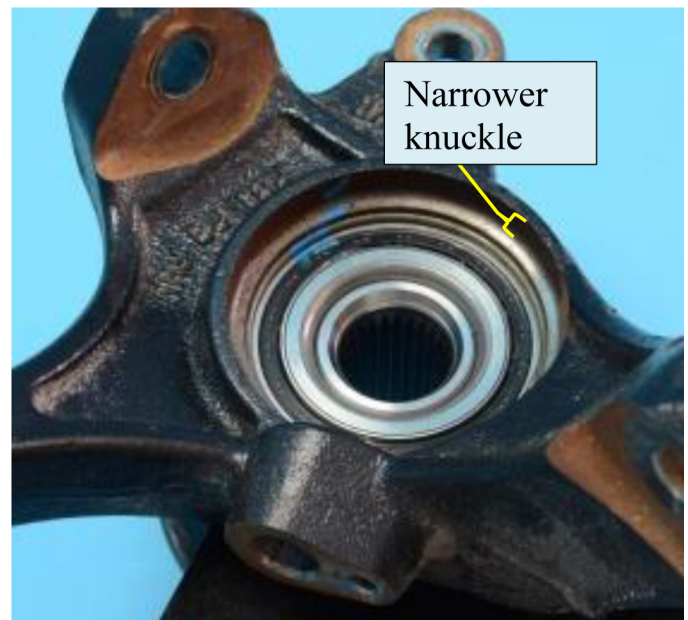
Figure 9. Wheel bearing and knuckle. The width of knuckle protection is narrower than figure 8 .
