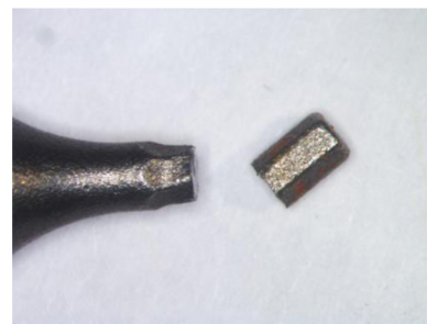
Figure 8. Fractured hex key
