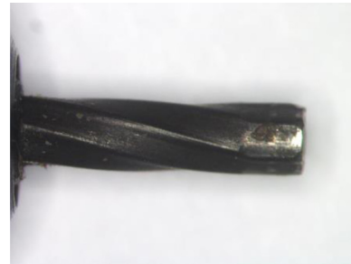
Figure 7. Twisted hex key
