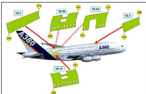
Figure 1. FML-shells produced by Premium Aerotec GmbH for A380
