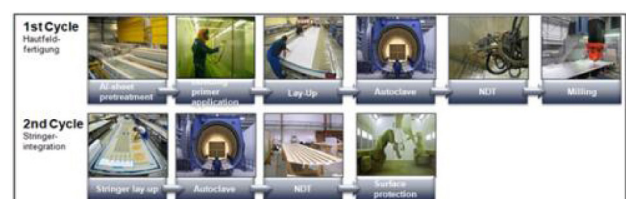
Figure 2. Process steps of the actual production
