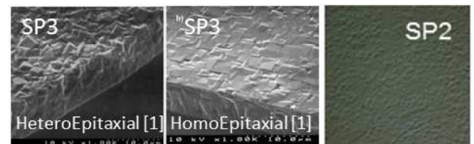
Figure 3. Characterization of Diamond Coating variations
