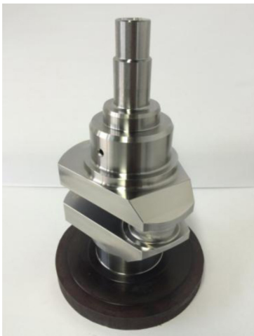
Figure 2. One of the machined billet crankshafts used in the engine. Three crankshafts were machined to provide strokes of 86, 98, and 115mm.
