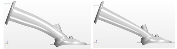
Figure 4. Intake port design for a Fill port (left) and a Tumble port (right).
