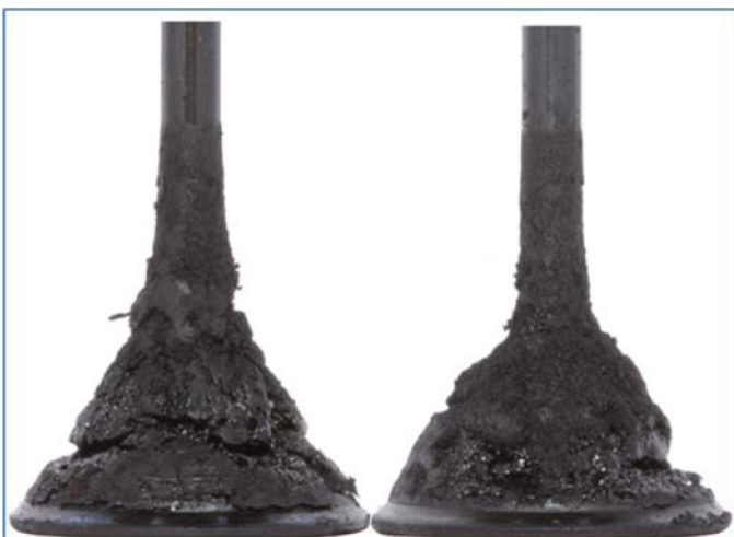
Figure 3. Ford Intake Valves After 190K km of Service
