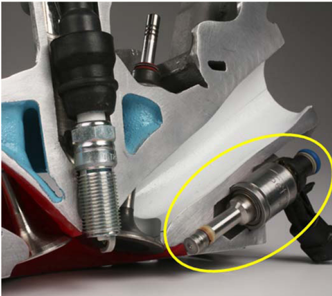
Figure 2. Cutaway Illustrating Direct Injection
