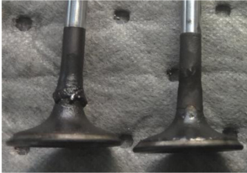
Figure 3. Hydrocarbon fouling on the back and stem of the intake valves due to liquid oil particles carried by blowby recirculation.
