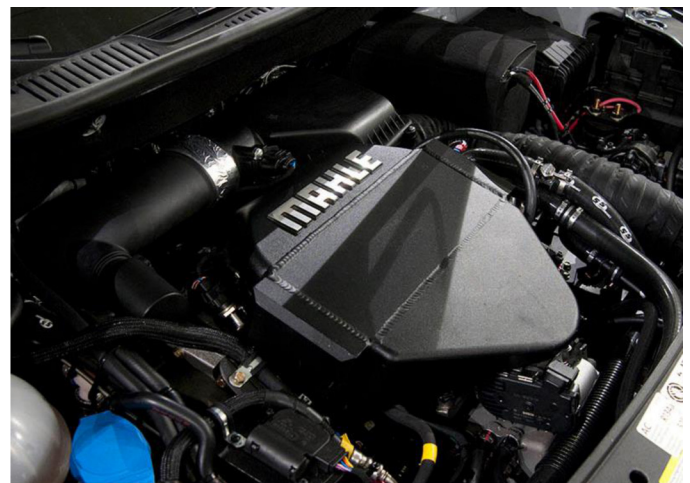
Fig. 1. MAHLE CNG Di3 engine installed in a demonstrator vehicle
