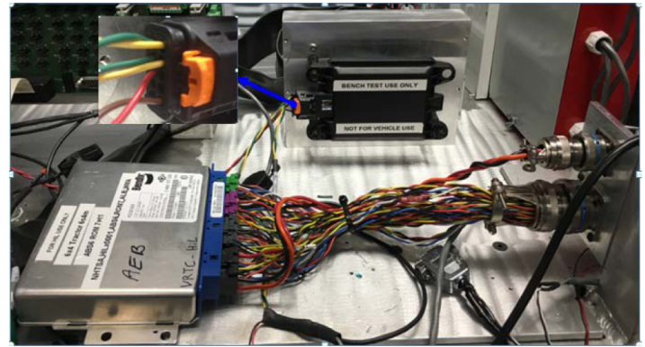
Figure 2. Bendix ECU and FLR20 radar on HiL system
