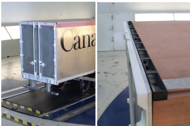
Figure 6. Trailer base details (left - lights and door hardware, right -rain gutter).
