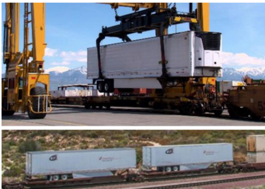
Figure 37. Unintended consequences -SmartWay trailers used on rail cars [14]
