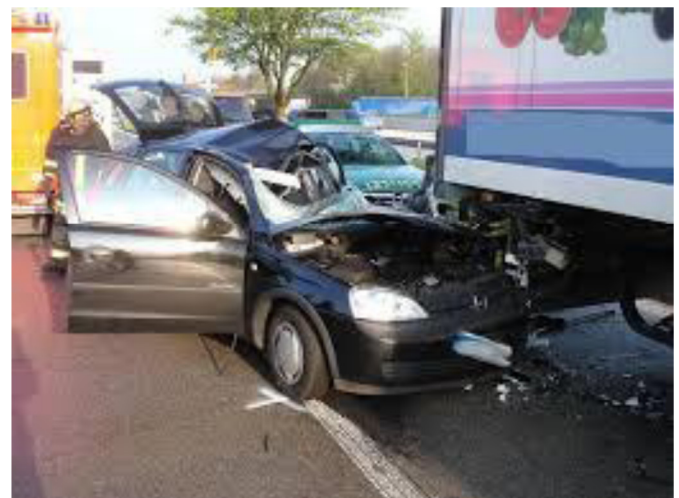
Figure 2. Car impacting rear side with rear under protection device
