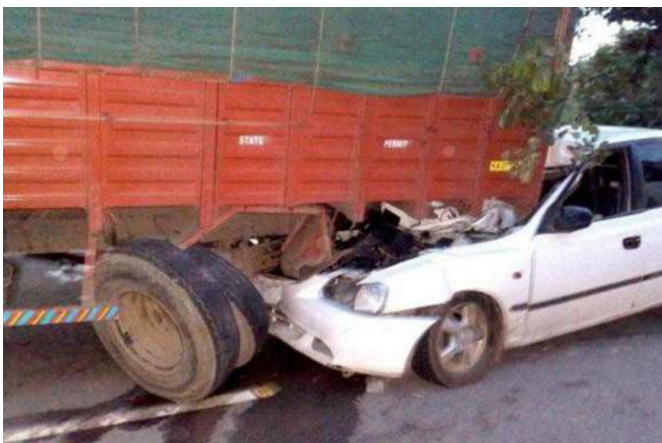
Figure 1. Car impacting rear side without rear under protection device
